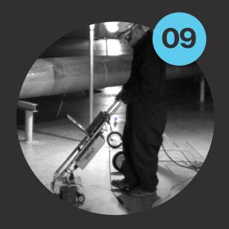
This technique relies on the principle of magnetizing the steel with a strong magnetic field generated by a powerful magnet. When the steel is in good condition, the magnetic field remains within the material.
