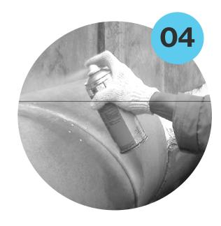
**Liquid Penetration Testing (DPI)**
